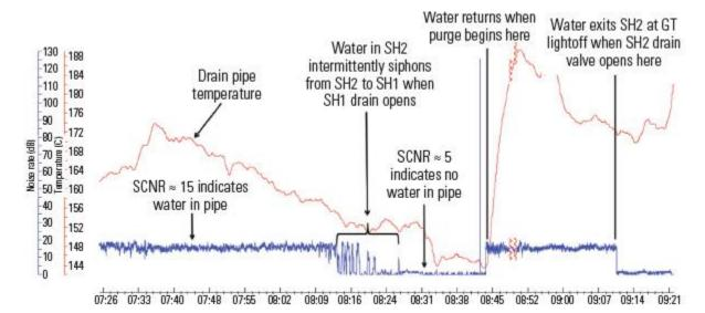
Steam or water? This graph shows activity inside the secondary superheater (SH2) drain pipe during a hot startup from 575 psig. The ultrasonic flowmeter equipment was monitoring but not controlling during this test. Source: FLEXIM Americas
