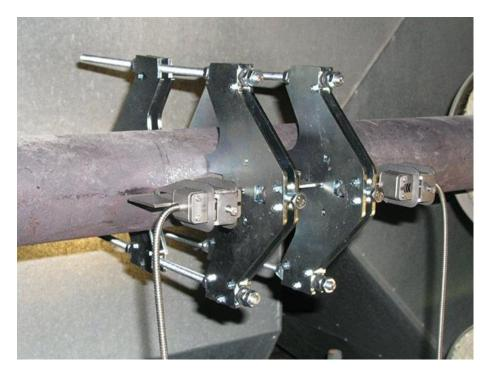
Innovative mounting feature. The WaveInjector fixture holds the ultrasonic flowmeter's transducers up to 4 inches off the pipe's surface, increasing the meter's operating temperature range to -260F to 750F. Courtesy: FLEXIM Americas
